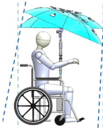
Figure 2: Proposed wheelchair attachment demonstrating tilt
