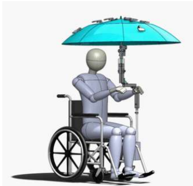
Figure I.14: CAD of full assembly showing load cell sensor placement, tilting, and stowing mechanisms
